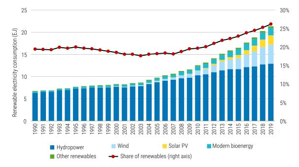
Figure 3.9 • Global renewable electricity consumption by technology, 1990-2019
